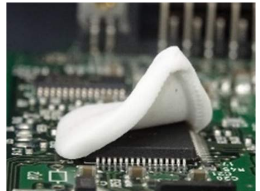
► Start of Development of a "Thermal Conductive Putty" Material Softer than Thermal Conductive Rubber
