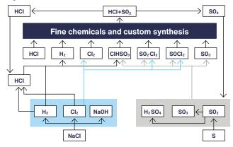
The CABB Group remains a pioneer in the circular economy. At its Pratteln site, the closed-loop system "Verbund System" enables highly efficient and sustainable chlorination and sulfonation reactions. Chlorine and sulfur trioxide are produced as primary raw materials and used to manufacture a variety of
