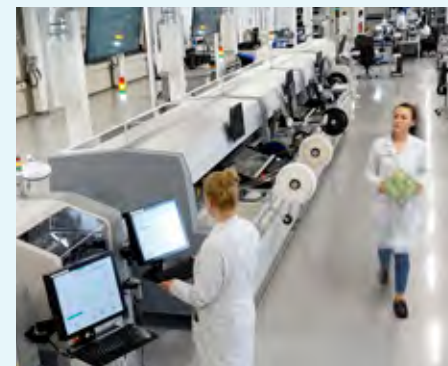
New full-line solution from Mycronic in action at Mikrolab, Germany, including two MY700 Jet Printers and three MY300 pick-and-place machines.
