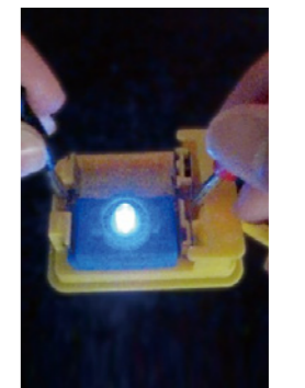
LED lighting that relies on a CNF-based electricity storage body
