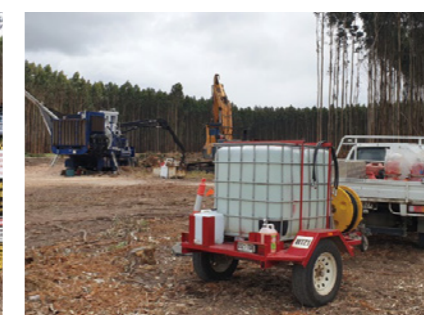
A portable firefighting system used for initial responses to fires
